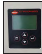
Under-counter main unit control panel
