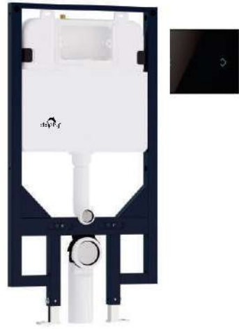
DTCC0004 Full Frame Concealed Cistern with Sensor Plate Leak Proof design Full Flush - 6L (Can be controlled to 4L) Half Flush - 3 L (Can be controlled to 2 L)
