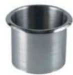
DWBN0010 Counter Top 304 Stainless Steel Diameter : Outside 160mm, Inside 140mm Chute Depth: 133mm
